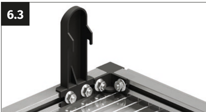
6.3 Press the anti-displacement device lightly against the rear plastic node and screw it in place using the two M6 flange nuts.
