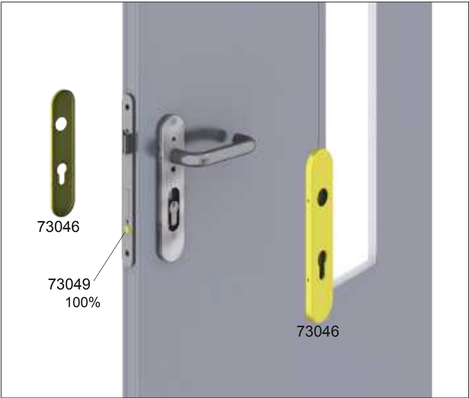
The Bolts (73049) should be fully tightened after install (73046) into (73043/73044)
