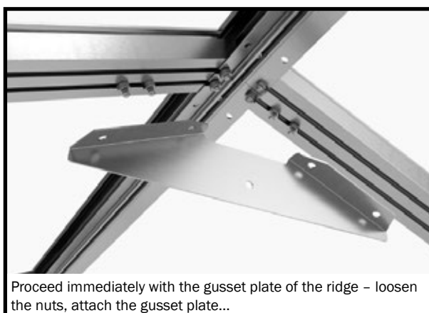
Remove the nuts from the screws inserted into the coupling profiles, position the screws corresponding to the holes in the gusset plate and place it on top.
