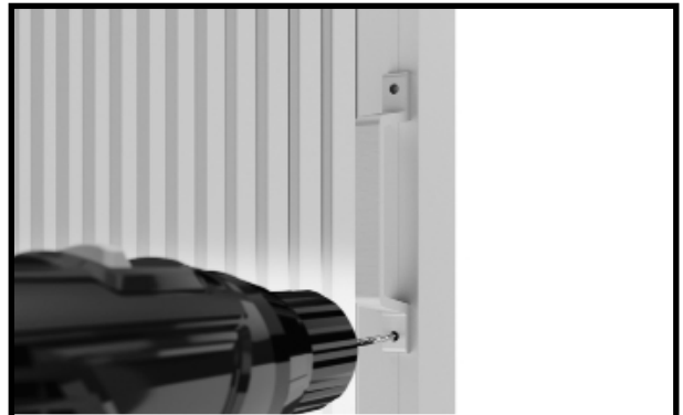
Pre-drill holes with a 4 mm drill bit.
